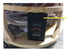
Re-assemble Ozone and insert the top screws.
