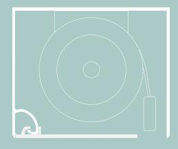
**Detachable cover** for later installation of blinds and access for maintenance.
