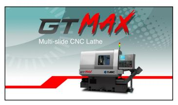
**GT Max:** Designed to replace the old Brown and Sharpe screw machines, the GT Max is a twin spindle gang tool lathe with 3 cross slides dedicated to the main spindle and a gang tool slide that can serve both the main spindle and sub-spindle. Using advanced CNC control, the main spindle can have up to 4 tools in the cut at the same time. The model series is available with bar stock capacity of 26, 36 and 43 mm.
