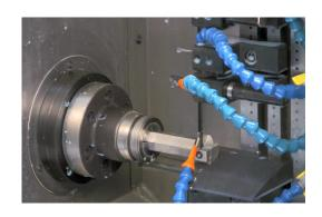
GTV series is a proven gang tool lathe platform for advanced operations such as hard turning, ramping, turn milling.
