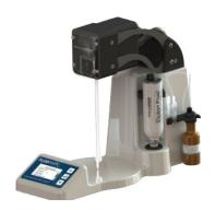
The concentration process uses tangentially-loaded, dead-end filtration to capture particles on porous membrane filters within the InnovaPrep CP's single-use tip. After the sample has been processed and the pathogens have been trapped, InnovaPrep's patented Wet Foam Elution™ process is employed to wash the pathogens off of the membrane surface into a very small liquid volume.
