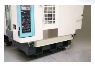
Optimized structure incorporates specially lightened vertical column and wide track design provides high dynamic characteristic able to accelerate quickly without vibration.
