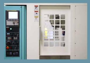
Operator control box can be swiveled for ease of use.
