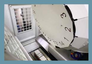
Pallet changer indexing is now based on an external encoder, which greatly raises positioning accuracy over the previous coupling gear based design.
