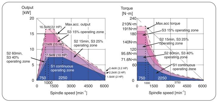
\* Charts for STS - 52J / STS - 60J would be slightly different due to pulley ratio of 1:2.45, instead of 1:2 on STS - 42J
